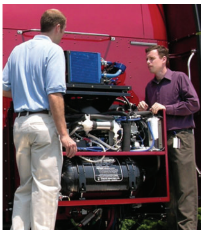
▲ Modine's idle-reduction system used a hydrogen fuel cell and carbon dioxide refrigerant to provide emissions-free cab heating/cooling but never got to market.
