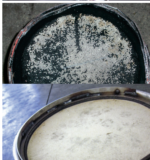
▲ Comparing the faces of a soot-fouled Diesel Particulate Filter and a professionally cleaned version.
