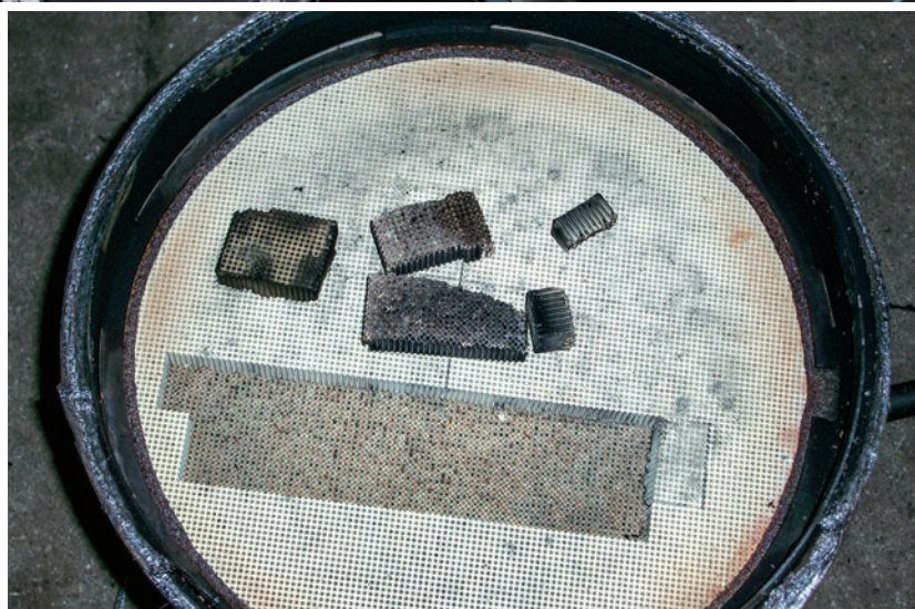
▲ A damaged Diesel Particulate Filter from the outlet side of the system. Note the plugging of the inner channels within the substrate.
